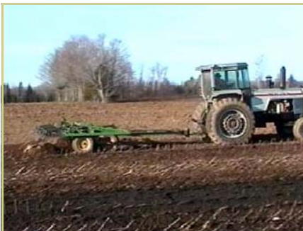
The Veazies use a soil saver to incorporate nutrients into the soil.
