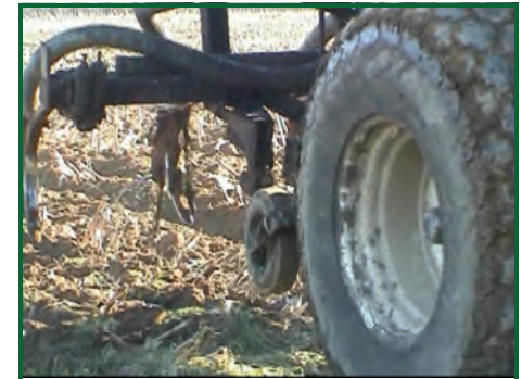
Roger has been experimenting with this injector that injects cow manure into the soil rather than on the surface.
