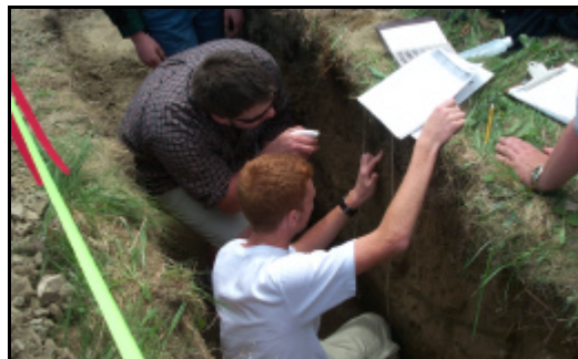
These students are trying to determine the horizon in this soil pit.
